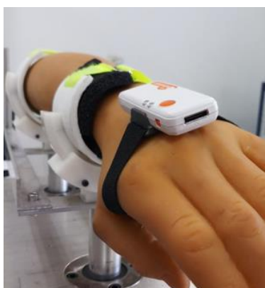
Figure 2: Shimmer device attached to hand model of test rig during testing
